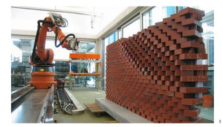
Figure 3: Programmed Wall, 5-axis robot building one of the wall scripts.
